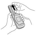
(1) To remove the cover, slide it outwards while pressing it down.
