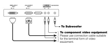
• If video equipment with an S video output terminal is used, connection with S video cable is recommended to provide finer video quality. (If the S-video input terminal and the video input terminal of AV3 connect to the monitor at the same time, S-video input would govern.)
