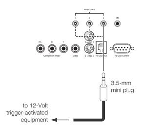
Figure 3-10. Connecting 12-Volt Trigger Outputs
