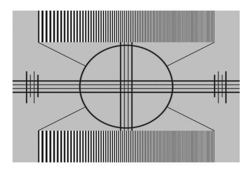
Figure 4-6. Typical Test Pattern for Adjusting Sharpness
