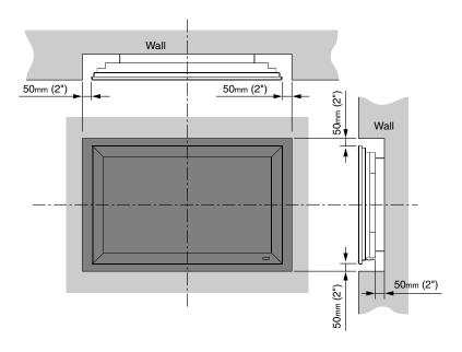
Figure 3-2. Ventilation Requirements for Enclosure Mounting
