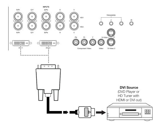
Figure 3-5. DVI Source Connections
