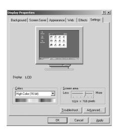
Click the **Advanced** button and click the **Monitor** tab on the dialog box. Set the vertical frequency to 60Hz and click **OK**.
