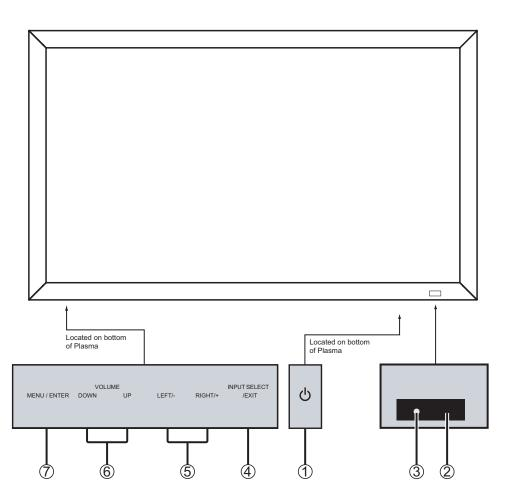
Figure 2-1. PlasmaWall Front-Panel Controls and Indicators
