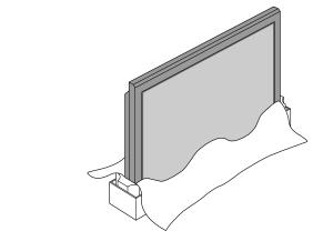
As it lies flat with the screen face down. Place the protective sheet, which was wrapped around the plasma monitor when it was packaged, between the screen and your work surface to avoid scratching or otherwise damaging the screen surface.
