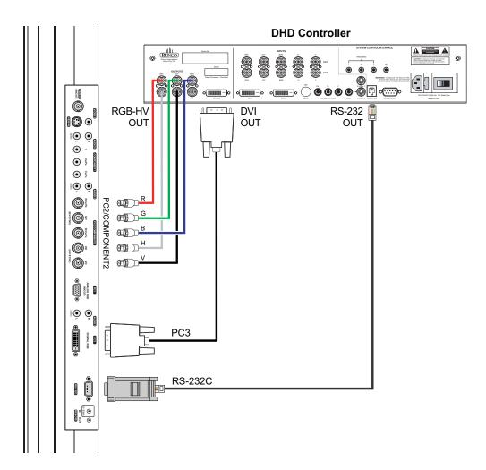
Figure 3-3. Connecting the PlasmaWall to the DHD Controller
