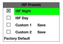
For each input, the PlasmaWall lets you save image quality settings as presets that you can recall at a later time. You can create up to four presets per input and resolution. Use the ISF Presets menu to recall saved image presets, or to save image settings in the "Custom 1" or "Custom 2" memory location. The currently-selected preset is indicated by a "\overline{\Omega}" to its left; in the example shown here, ISF Night is selected.
