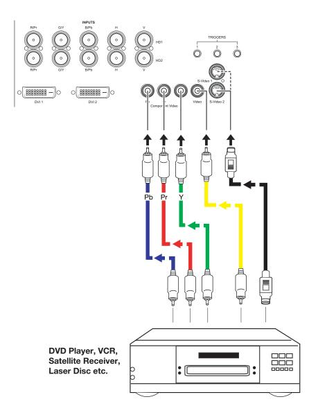
Figure 3-8. Composite, S-Video and Component Video Connections
