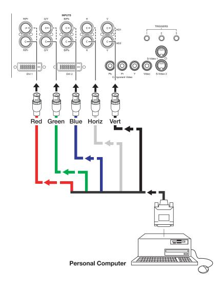
Figure 3-7. Analog RGB Connections
