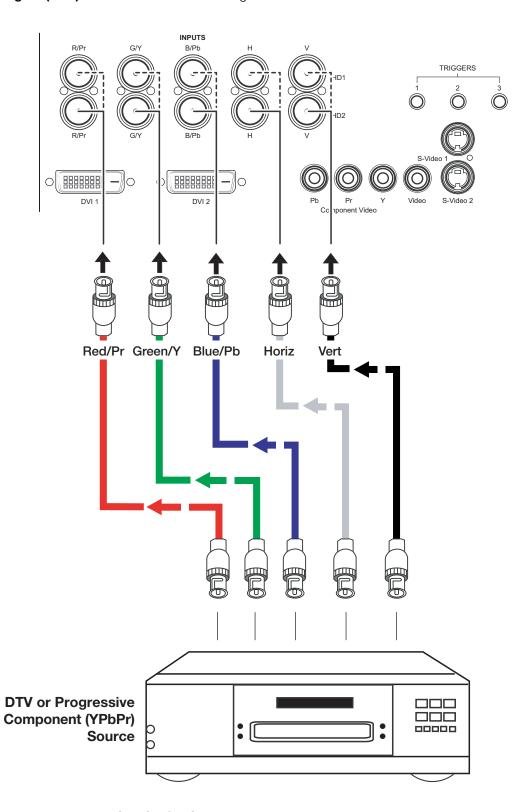
Figure 3-6. Digital (DTV) RGB Connections
