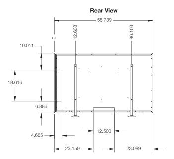
Figure 7-1. PlasmaWall Model PL-61DHD Dimensions
