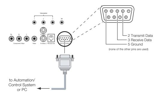
Figure 3-9. RS-232 Control System Connection
