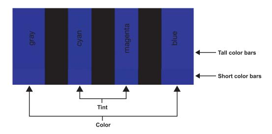
**Tint:** Tint or "hue" is essentially the ratio of red to green in the color portion of the image. When tint is decreased, the image appears redder; when it is increased the image appears greener. To set the tint, select Tint and press **ENTER**. While looking at the color bar pattern through a blue filter, adjust the tint level until the cyan and magenta color bars (on either side of the green bar) appear to be a single shade of blue.
