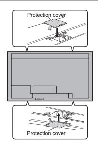
After installing the monitor, affix the protection covers (4 pieces) as necessary.
