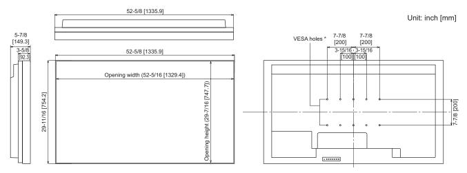
When mounting the monitor, be sure to use a wall-mount bracket that complies with the VESA-compatible mounting method. SHARP recommends using M6 screws and tighten the screws.
