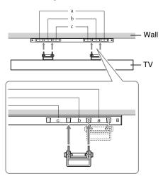
**5** Adjust the angle of the Mounting Hook.
