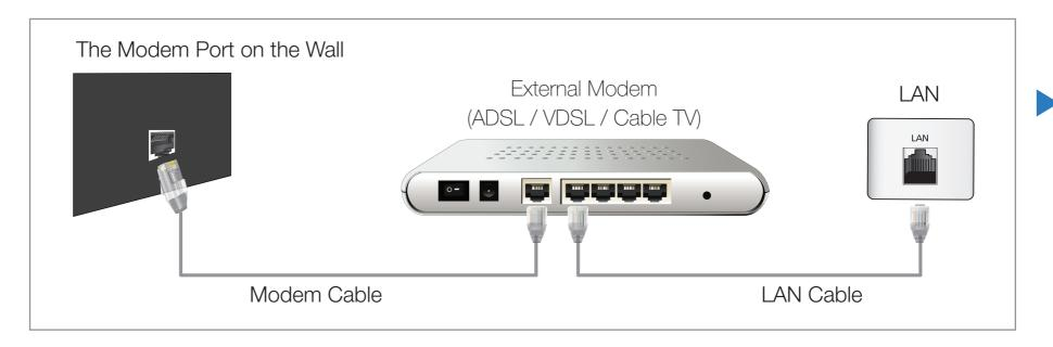
You can attach your TV to your LAN by connecting the LAN port on the back of your TV to an IP Sharer which is connected to an external modem. Use LAN cable for the connection. See the diagram below.
