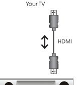
With an HDMI ARC setup, the audio connection between your TV and Home Audio Receiver can be removed. The HDMI cable will transmit audio signal to and from your TV with an all-digital audio/video connection.
