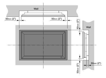
Figure 3-2. Ventilation Requirements for Enclosure Mounting
