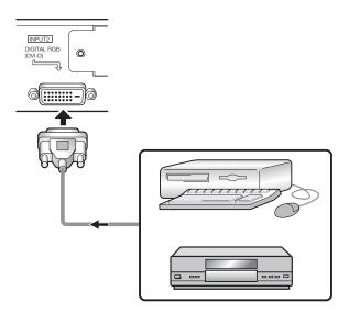
Figure 3-5. DVI-D (INPUT 2) Connection
