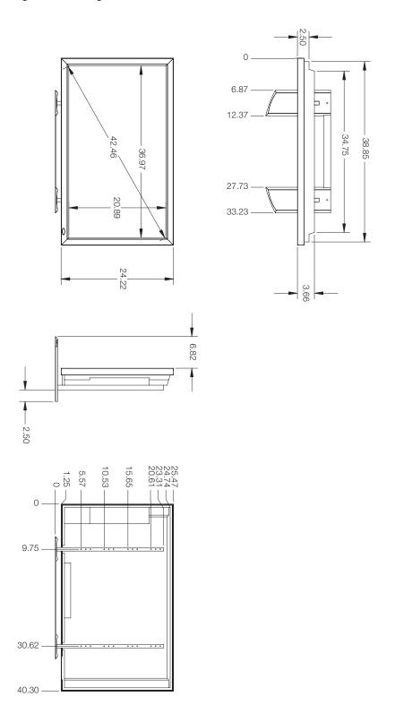
Figure 7-1. PlasmaView Model VP-4200 Dimensions (with Optional Table Stand)
