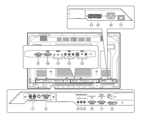
Figure 2-2. PlasmaView Model VP-4200 Connector Panel
