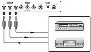
Figure 3-10. Connecting Audio Inputs
