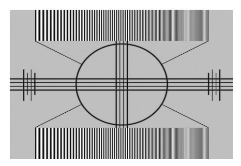
Figure 4-6. Typical Test Pattern for Adjusting Sharpness
