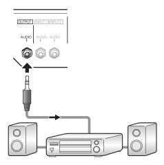
Figure 3-11. Audio Output Connection
