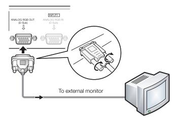
Figure 3-4. ANALOG RGB OUT (INPUT 1) Connection
