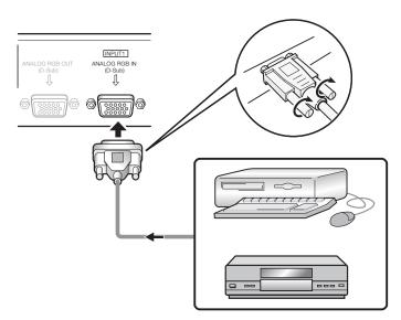
Figure 3-3. RGB/Component Video (INPUT 1) Connection
