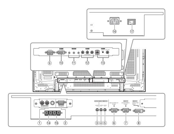
Figure 2-3. PlasmaView Model VP-6000 Connector Panel
