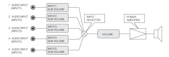
Figure 4-7. Audio System Functional Block Diagram
