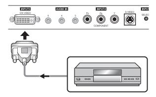
Figure 3-8. DVI-D (INPUT 5) Connection
