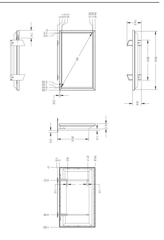
Figure 7-2. PlasmaView Model VP-6000 Dimensions (with Optional Table Stand)
