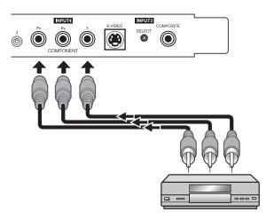
Figure 3-7. Component Video (INPUT 4) Connection
