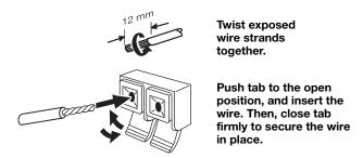
Figure 3-12. Connecting Speakers
