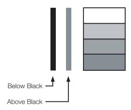
Figure 4-3. Typical PLUGE Pattern for Adjusting Brightness
