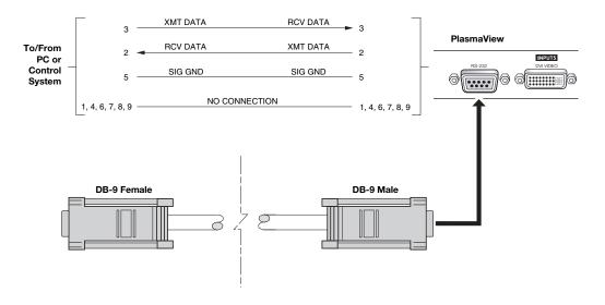
Figure 3-13. RS-232 Control System Connection
