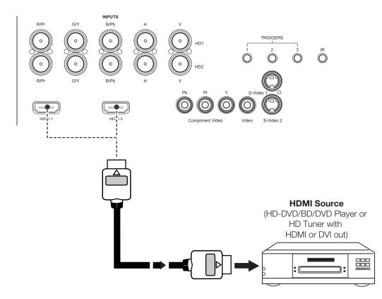
Figure 3-5. HDMI Source Connections
