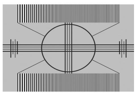
Figure 4-5. Typical Test Pattern for Adjusting Sharpness
