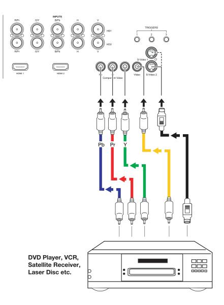
Figure 3-8. Composite, S-Video and Component Video Connections
