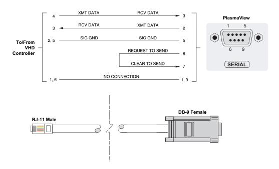
Figure 3-4. RS-232 Connection from the VHD Controller to the PlasmaView
