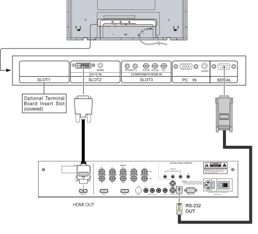
**Digital Video Connection:** The PlasmaView has a DVI input, labeled **DVI-D IN (SLOT 2)**. Connect the HDMI output from the VHD Controller to this input, using a DVI-to-HDMI cable or a DVI cable with a DVI-to-HDMI adapter.
