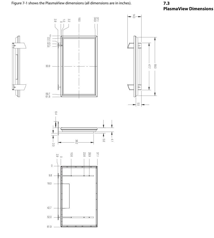
Figure 7-1. PlasmaView Model VP-6500VHD Dimensions (with Optional Table Stand)
