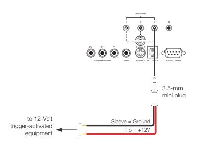
Figure 3-10. Connecting 12-Volt Trigger Outputs
