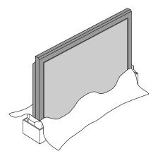
As it lies flat with the screen face down. Place the protective sheet, which was wrapped around the plasma monitor when it was packaged, between the screen and your work surface to avoid scratching or otherwise damaging the screen surface.
