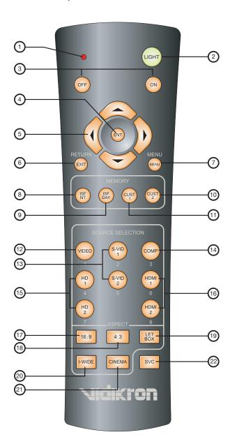
Figure 2-5. VHD Controller Remote Control
