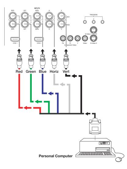
Figure 3-7. Analog RGB Connections
