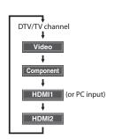
Pressing [CHANNEL —] reverses the direction of the input modes.
