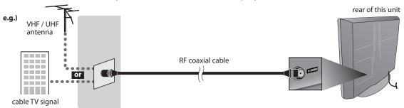
\* Once connections are completed, turn on the unit and begin initial setup. Channel scanning is necessary for the unit to memorize all available channels in your area. (Refer to "Initial Setup" on page 15.)
