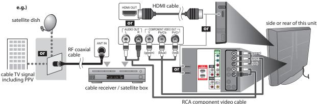
\* You can also connect this unit to the cable receiver or satellite box other than the HDMI or the component video output jack because they might have different output jacks.
