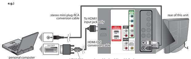
HDMI-DVI conversion cable should be with ferrite core.
