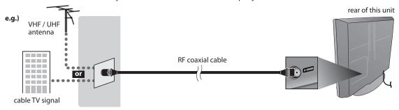
\* Once connections are completed, turn on the unit and begin initial setup. Channel scanning is necessary for the unit to memorize all available channels in your area. (Refer to "Initial Setup" on page 13.)
