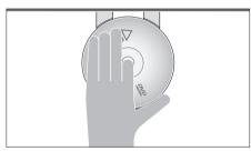
Place a disc in the loader with the label facing upwards. Eight centimetre discs may only be loaded provided with a suitable adaptor. Discs of other shapes cannot be played.
