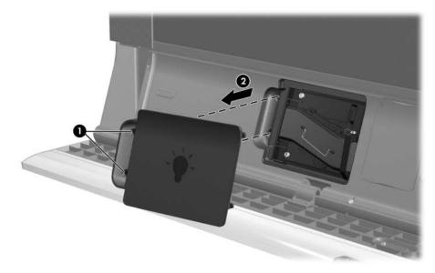
5. Loosen the three screws ① on the lamp module; then pull out the module using its handle @.
