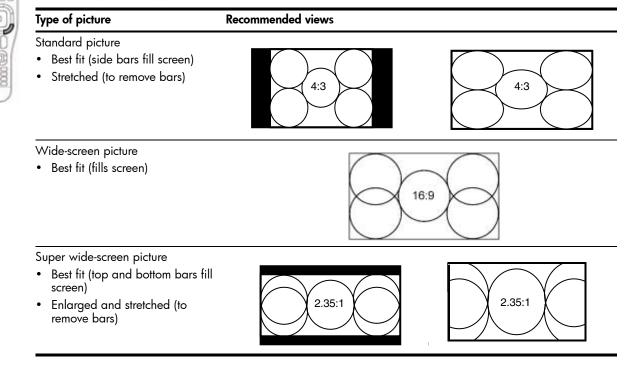
**TIP:** If you can set the video output from a source device to have 16:9 aspect (wide-screen picture), you should select that setting. Refer to the instructions for the video device. This provides maximum compatibility between the device and the TV.
