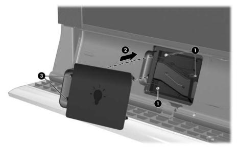
8. Plug in the power cord and turn on the TV. If the lamp does not turn on after the warm-up period, reinstall the lamp module.
