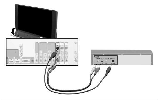
**NOTE:** You can connect to the Video 1, Video 2, and Video 3 inputs on the TV. Only one S-video or composite-video connection is supported for each of these three inputs.
