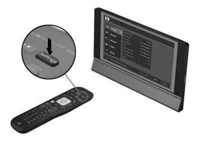
**NOTE:** You can use the buttons on the side of the TV to work the on-screen menu:
