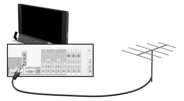
**TIP:** If your antenna has flat, twin-lead cable or other type of cable, connect the antenna cable to a coaxial adapter; then connect the adapter to the TV antenna input.
