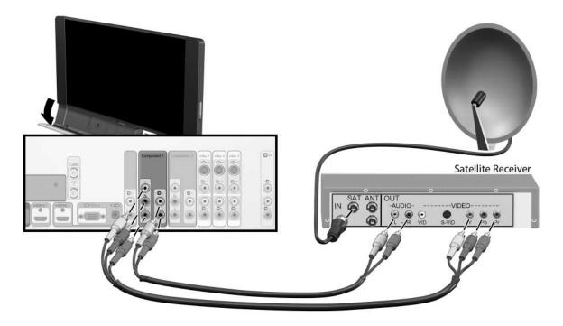
**NOTE:** If your device has different connectors from those shown, use the highest quality video connection available. Observe the color-coding on connectors.
