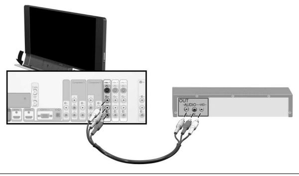
**NOTE:** You can connect to the Video 1, Video 2, and Video 3 inputs on the TV. Only one S-video or composite-video connection is supported for each of these three inputs.
