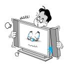
When moving the TV assembled with speakers do not carry holding the speakers.
