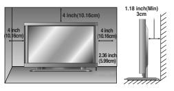
Table stand mount minimum allowable clearances for adequate ventilation.
