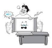
When installing the TV on a table, be careful not to place it too close to the edge of the table.
