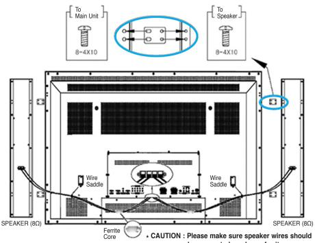
Please make sure speaker wires should be connected as above, ferrite core are to be nearer to the main unit not to speakers to avoid possible electromagnetic-interference.
