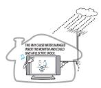
Bend antenna cable between inside and outside building to prevent rain from flowing in.
