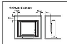
If the television is to be built into a compartment or similar enclosure, the minimum distances must be maintained. Heat build-up can reduce the life of your television, and can also be dangerous.
