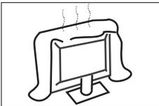
Do not block the ventilation holes on the back cover of the TV. Adequate ventilation is essential to prevent failure of electrical components.
