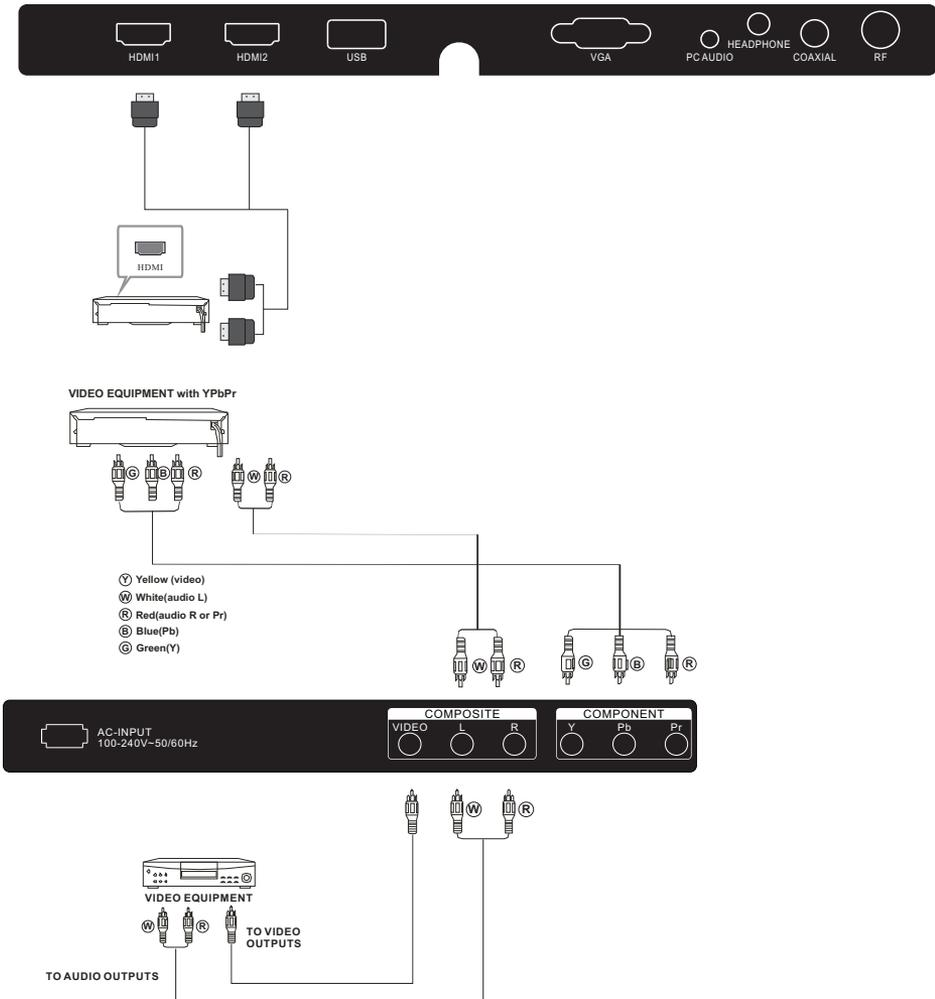
The television's inputs can be connected to the following types of equipment: VCR, multi disc player, DVD, camcorder, video game or stereo system, etc.....
