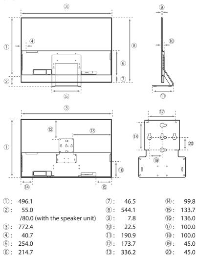
$lue{}$  Use screws of adequate length (M4  $\times$  12 – 16) to fix the VESA bracket and wall mount adapter.
