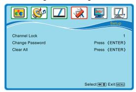
**Channel Lock:** To lock channels. Use **◄►** to select the channel you want to lock, and then press **ENTER** to lock or unlock it.
