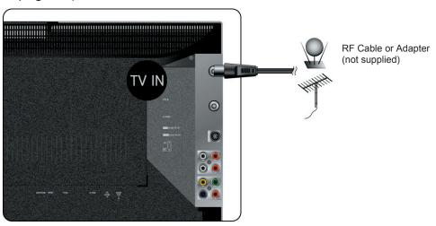
2) DTV: Connect the LCD TV to the cable with DTV signals and preset DTV channels into memory with AUTO SCAN function in DTV menu (see page 21).
