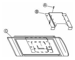
Follow these steps to attach the wall mount. (Screw: M10 x 4; Screw bolt 3/8 inches x 6)
