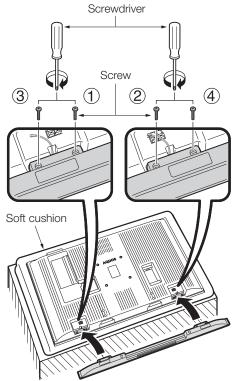
Insert and tighten the 4 screws with the hex key (supplied with the product) in the order of (1), (2), (3) and (4).
